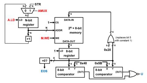
Inputs for use by external logic, including the STR input, are shown in black. Datapath control signals appear in red. Datapath outputs are shown in blue.
