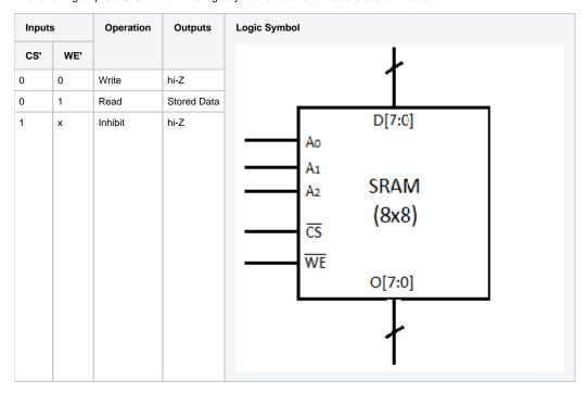
$A_0$ - $A_2$  are the address lines,  $D_0$ - $D_7$  are the data lines, and  $D_0$ - $D_7$  are the data outputs. The outputs are gated with tri-state buffers and are in the high impedance (hi-Z) state whenever the Chip Select (CS') input is 1. They are available only in the Read mode. Chip Select (CS') and Write Enable (WE') inputs are <u>activeLOW</u>.
