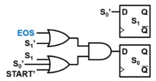
a) The system starts in a WAIT state  $(S_1S_0=01)$ , allowing external logic to write a string into the memory (logic not shown). The external logic provides the starting address of the string through the STR input and raises the START input to make the FSM change any upper-case letters in the string to lower case.
